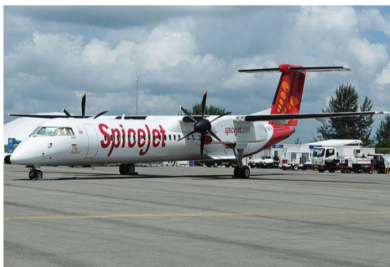
Figure 06 : A Q400. Note that the horizontal tail is mounted high up on the vertical one, and not at the fuselage level as in Our Plane and most jetliners. The image [01] carries the appropriate permissions for this usage.
