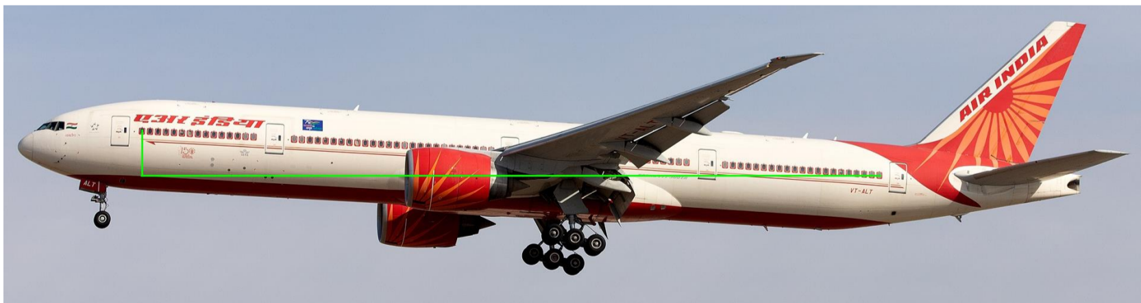
Figure 13 : The aircraft from Q01 of the Quiz. Relative to the horizontal (green line), the d-axis (along the windows) is raised by approximately 75 pixels for 1240 pixels' horizontal run, giving a pitch of 3^\circ .
