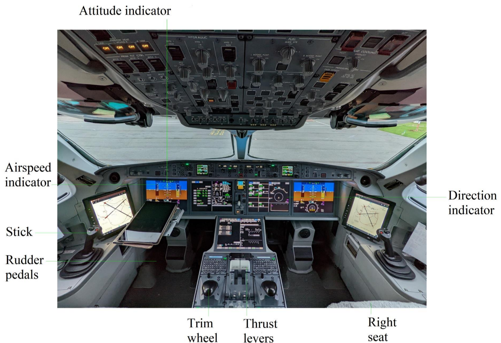
Figure 06 : A picture of a cockpit with salient parts labelled. The aircraft is a Bombardier C-Series, later known as Airbus A220. The image [01] carries appropriate permissions for this usage. I did not find a picture of a 'more standard' airliner cockpit which can be used as a demonstration and also carries the suitable permissions.
